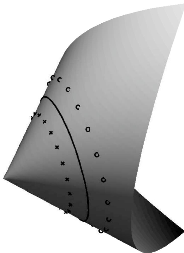
*Figure 4.* The crosses and circles from Figure 3 can be mapped to a three-dimensional space in which they can be separated by a linear perceptron.
